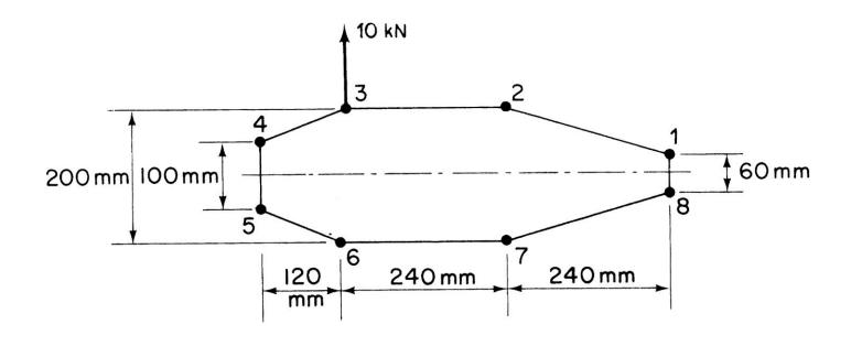
FIGURE 20.11 Closed Section of Beam of Example 20.4
