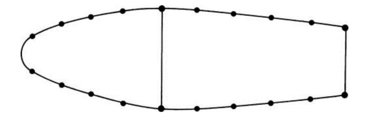
FIGURE 20.2 Idealization of a Wing Section
