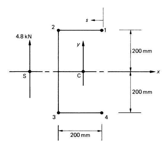
FIGURE 20.7 Idealized Channel Section of Example 20.3
