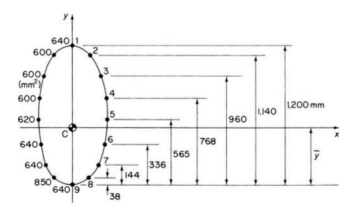
FIGURE 20.5 Idealized fuselage Section of Example 20.2
