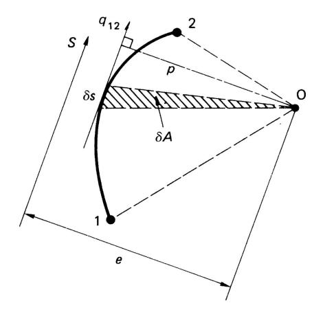
FIGURE 20.10 Moment Produced by a Constant Shear Flow
