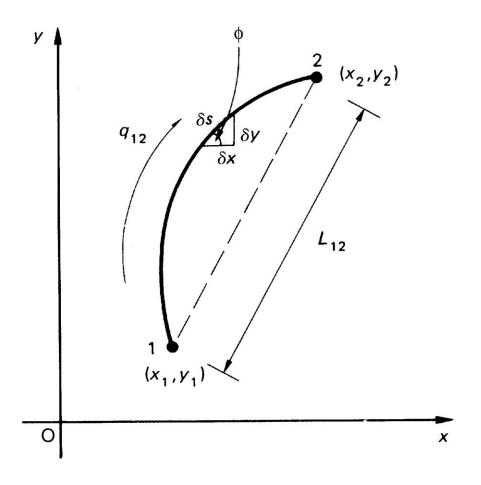
FIGURE 20.9 Curved Web with Constant Shear Flow
