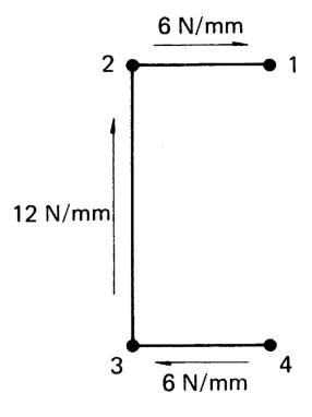
FIGURE 20.8 Shear Flow in Channel Section of Example 20.3
