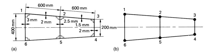
FIGURE 20.4 Idealization of a Wing Section
